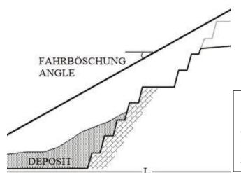
**Figure II\_C** – An example of landslide runout and deposit area of potential geohazards on Site based on simplistic Farböschung assessment.
